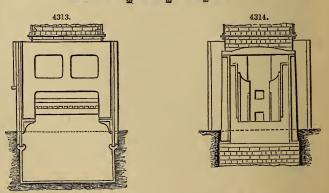
especially at the end next the stack, where the general rule is to have the under side of the arch level with the lower side of the doorway.
